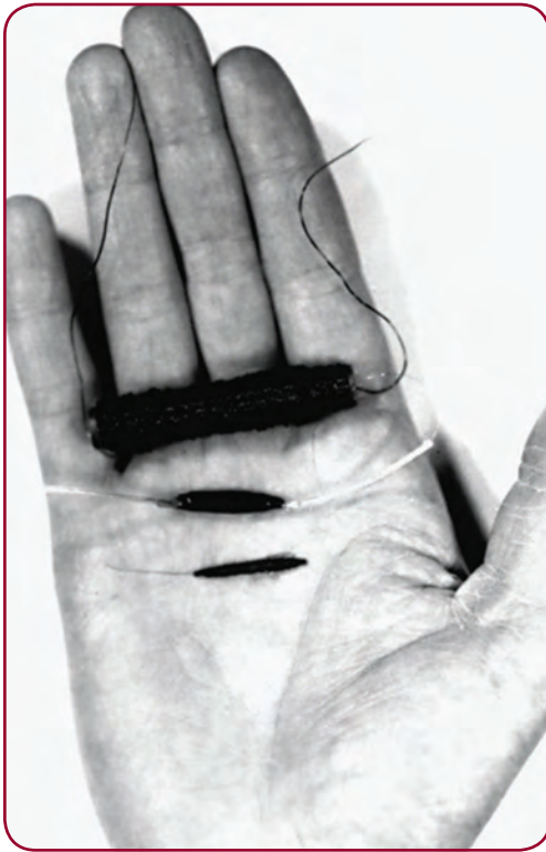
FIGURE 1–8. An example of induction coils used by Charles Eyriès and André Djournio. Image provided courtesy of Claude-Henri Chouard, M.D.
