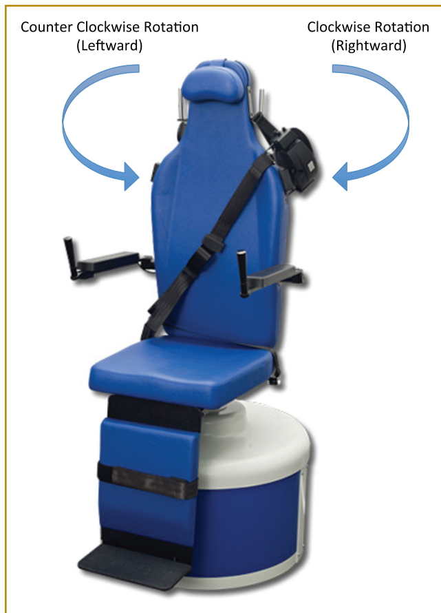
FIGURE 6–1. Rotational chair showing direction of clockwise (rightward) and counterclockwise (leftward). Image courtesy of Micromedical, Inc.
