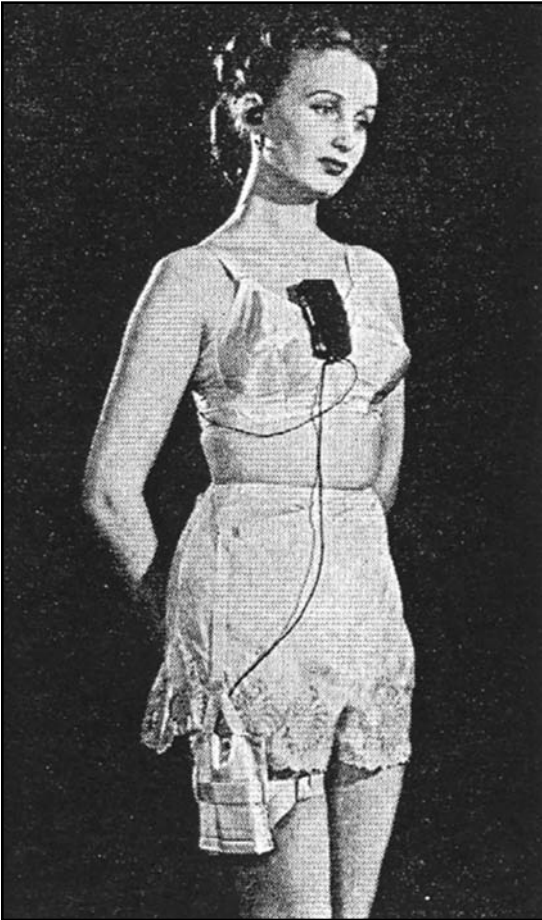
Figure 6-1. How a hearing aid was worn in the 1930s. The amplifying unit, mounted on the chest, was supplied by batteries strapped to one leg, and was connected by a long, flexible wire to the transducer mounted in a fully occluding earmold. (Reprinted from Hearing and Deafness , first edition, Murray Hill Books, 1947.)
